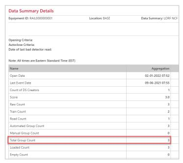
The LORF NCF Alert coincides with an update to Rule 3 of the AAR Field Manual giving handling carriers cause to shop a car with an open LORF NCF Condemnable alert. This alert can be interpreted to mean that the given piece of equipment has a high probability of having some brake defect related to LORF NCF.
